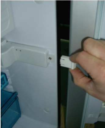
1. Locate the thermostat housing inside the fridge and remove the light button
