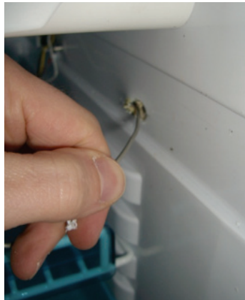
7. Carefully remove the thermostat capillary probe
