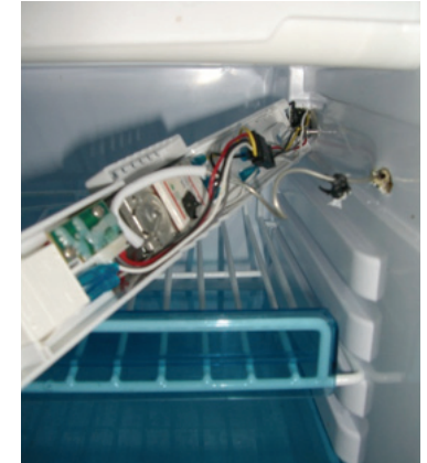
5. Pull the thermostat housing forward. It should now come away from the wall
