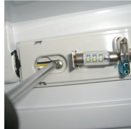
4. Loosen the rear screw, this doesn't have to be removed
